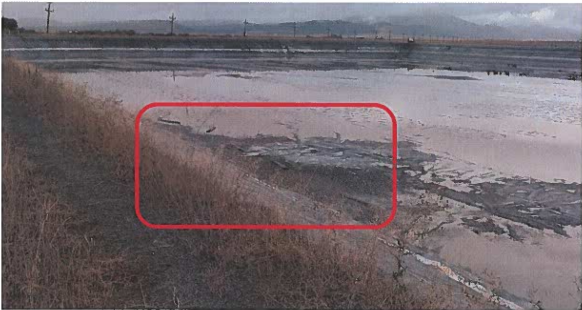
Figure 3: Ballasts lying along the edge of the south pond perimeter on October 4, 2018.
